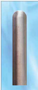
UCV/B/205 Dome top Material: s. steel Finish: satin Height: 1000mm Planted: 300mm Diameter: 150mmø
